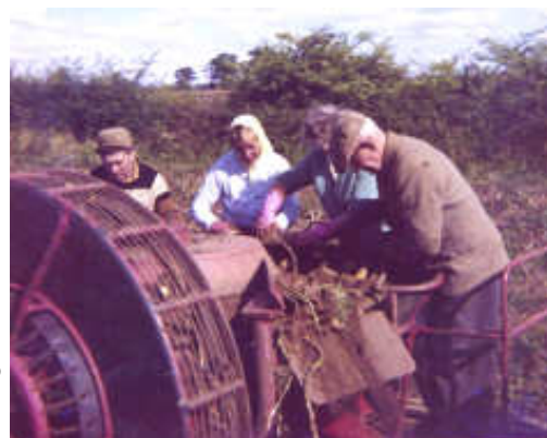
Massey Ferguson spud harvesters suffered from not having enough room on the circular table to pick all the potatoes off before the spoil was returned to land, this resulted in some of the crop being lost!
