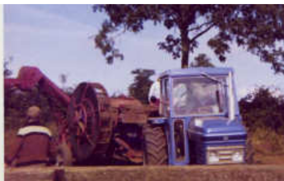
Later on we bought a new Leyland 384 and a second-hand Ferguson potato harvester, also a single row machine but this time it was a bulker. These harvesters required three hydraulic tappings on the tractor.
