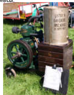
Peter Foster's 1933 Villiers 1.5hp. The only stationary engine that Villiers produced, it was well received by small power users as it was reliable and economical.
