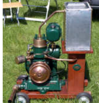
Peter Foster's 1933 Villiers 1.5hp. The only stationary engine that Villiers produced, it was well received by small power users as it was reliable and economical.
