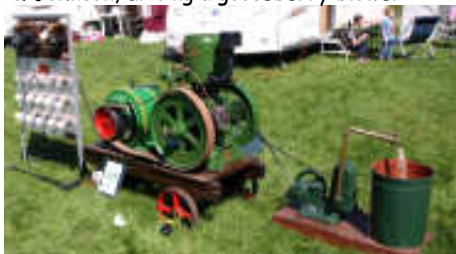
Owned and restored by A.Oglesby a 1926 2hp Waugh & Josephson a copy of a Fuller & Johnson, driving a gooseberry blower
