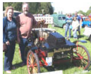
Completely original 1902 Bartholomew owned for 7 years by Colin Klyn. Built for a horse and later converted with an engine. It's the only one in existence, top speed 12 mph, 20/25 mpg. They have completed the London to Brighton Run once, after 6 attempts.
