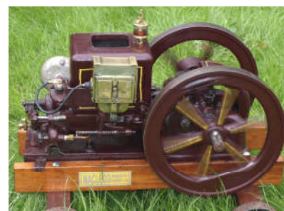
A rare 1926 Macleod 1.75hp owned by Cliff Smith. This was a 'basket case' and has been restored, new parts, re-assembled and painted over the last 2 years.
