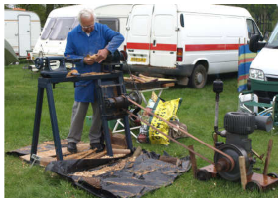
Ted Maile working at his lathe powered by a Wolsely engine producing beautiful pieces of woodwork.
