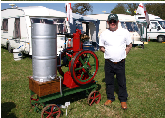
Left: A rare 1919 Pilter made by American Stover Co. Dick Culley bought it as a basket case and restored it to present condition. He then sold it to Sid Banham. Used to drive various farm machinery.
