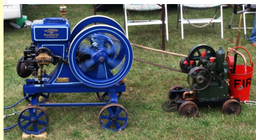
Shane Marrows had 2 displays, a 1927 Lister L and as shown below a 1945 Lister Start-O-Matic, a lighting plant of 240 volts output
