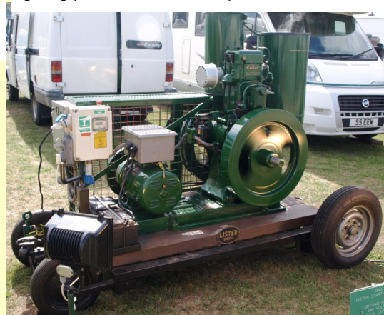
Shane Marrows had 2 displays, a 1927 Lister L and as shown below a 1945 Lister Start-O-Matic, a lighting plant of 240 volts output
