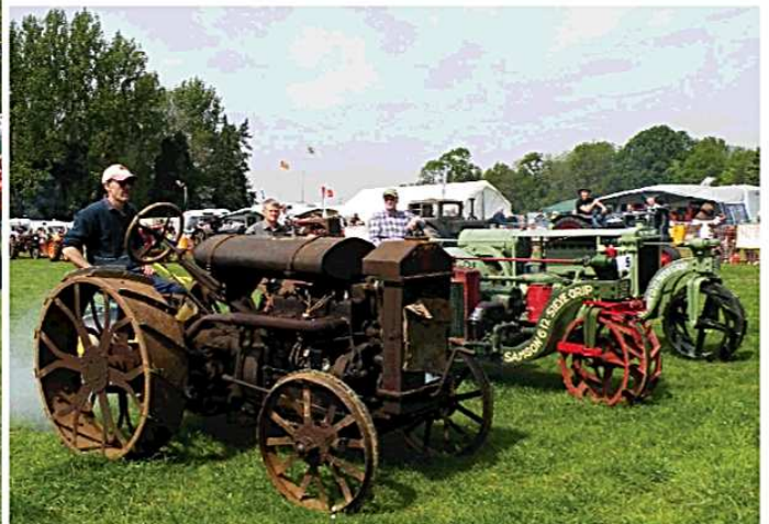
Three Samson's in a row, possibly for the first time in this country Allan Sale's 1920 Samson model M 4 cylinder 2 speed, Bryan Beba and Gordon Carson's 1917 model 6-12 single cylinder straight petrol then Gerald Gregory's 1916 Sieve Grip model 12-25
