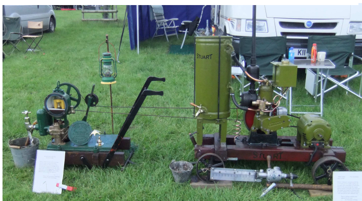
Above: Stacey & Lisa Burnett have owned this 1920 Fairbanks Morse, model ZA 1.5hp for 2 years. It once worked daily at a blacksmiths on a farm with the Newman family until the 1970's when it was put into storage but started up regularly before being sold to an enthusiast. The model ZA was in production from 1915-46. Shown here running a Lister H3 pump.
