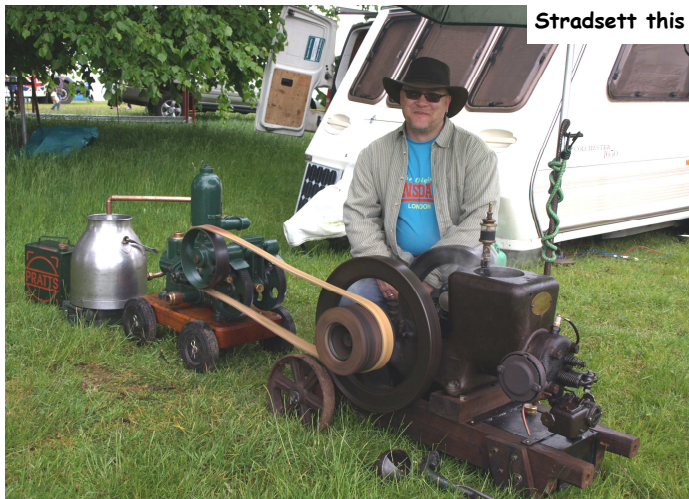
Above: Stacey & Lisa Burnett have owned this 1920 Fairbanks Morse, model ZA 1.5hp for 2 years. It once worked daily at a blacksmiths on a farm with the Newman family until the 1970's when it was put into storage but started up regularly before being sold to an enthusiast. The model ZA was in production from 1915-46. Shown here running a Lister H3 pump.
