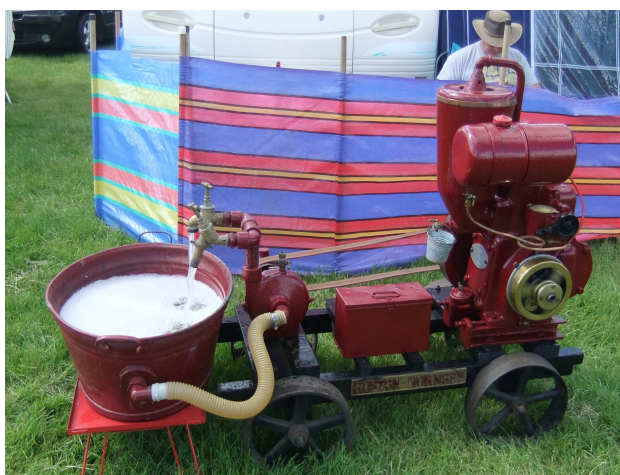
Below: 1936 Ruston Hornsby PT Carrot Top owned by Mr Richard Tinkler for 33 years and previously worked pumping water from a canal to a cattle trough.
