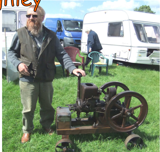
Above: Owned by G. Pearson for the last 10 years this 1920 Amanco Hired Man 2.5hp is all original except for the fuel tank,
