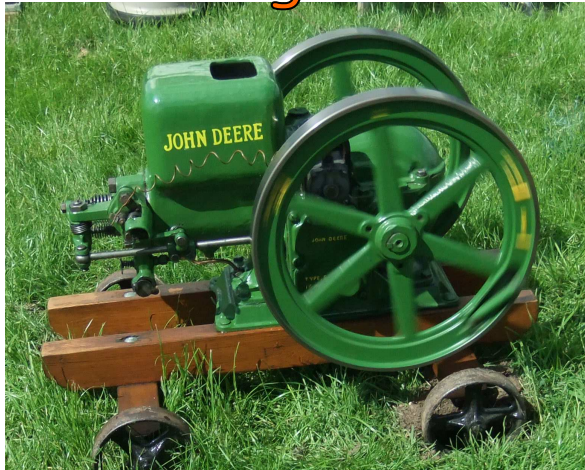
Above: 1929 John Deere E 1.5hp owned by Cliff Smith. Originally from USA it was used to power water pumps and milking machines
