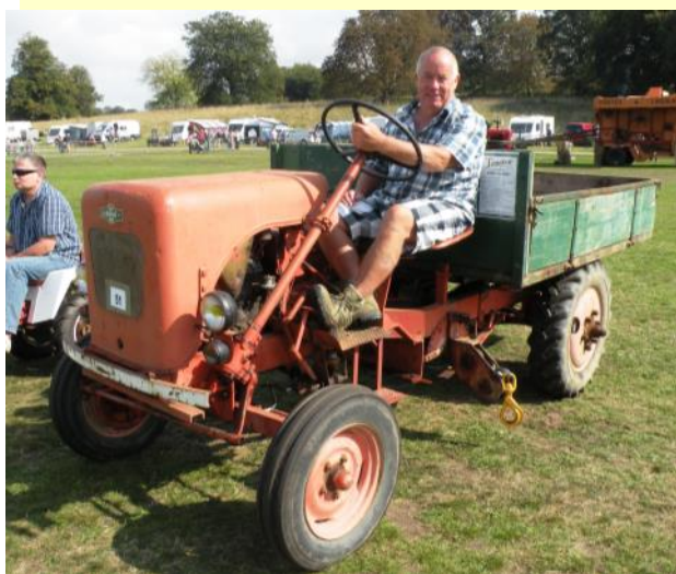
Left: Mr Peter Dolman with his Burwell 1965 Benetulliere Multi-plex 412 which was designed and built in the vineyards of the Beaujolais region of France. The side winch enabled hand steered implements to be pulled up the steep slopes between the rows of grape vines. This particular model was powered by a Renault 8
