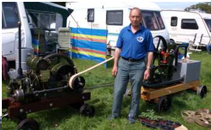
Right: Owned by Matt Reading this 1943 6.5hp Lister LHM made its rally debut this year at Stradsett. The engine was purchased in 2014 after 40 years of storage in North Yorkshire. It was supposed to be hopper cooled but had been converted at some point to being tank cooled. Matt, together with Scott and Simon made a steel trolley and converted the engine to being screen cooled with the addition of a Stuart Turner pump. It was shown driving a R. Hunt No 2 combined crushing and driving mill that came from a farm in Mayland on Sea, Essex. It had been stored outside due to the farm changing from crops to cattle and was totally seized. It also had some frost damage. It was completely dismantled and overhauled in winter 2014/15 and made ready for flour making at Stradsett this year. Paintwork by Kirsty.
