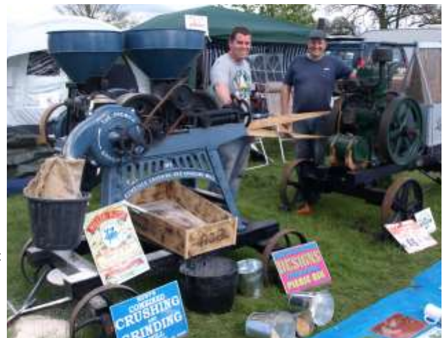
Right: Owned by Matt Reading this 1943 6.5hp Lister LHM made its rally debut this year at Stradsett. The engine was purchased in 2014 after 40 years of storage in North Yorkshire. It was supposed to be hopper cooled but had been converted at some point to being tank cooled. Matt, together with Scott and Simon made a steel trolley and converted the engine to being screen cooled with the addition of a Stuart Turner pump. It was shown driving a R. Hunt No 2 combined crushing and driving mill that came from a farm in Mayland on Sea, Essex. It had been stored outside due to the farm changing from crops to cattle and was totally seized. It also had some frost damage. It was completely dismantled and overhauled in winter 2014/15 and made ready for flour making at Stradsett this year. Paintwork by Kirsty.
