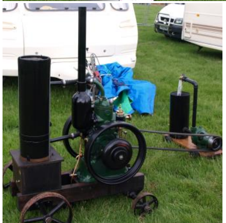
Centre: Dennis Andrew's 1917 Ingeco Type W 3hp owned for 6 years. It was in an old building in Grantham and he received it in payment for helping to clear a shed out. It took 1 year to restore with new parts being made. See picture of unrestored state.
