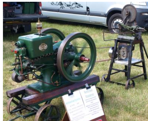
Graham Turner's 1922 International Harvester M Type 3hp bought in 1995 and restored by Graham. Driving a Band Saw Sharpener.
