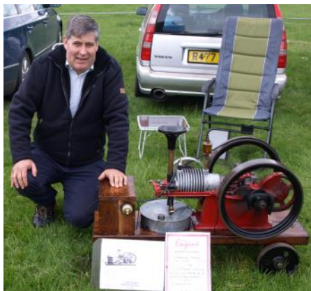
Left: Michael Atkin with his 1914 International Harvester Tom Thumb 1hp fitted with optional slow speed pulley for driving a cream separator.
