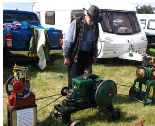
Barry Burden's 1924 Fairbanks Morse Z Type 'Dishpan' 1.5hp driving a Petter A2 cutaway engine finished to this stage to show the workings of an engine. Left: This small 2 stroke engine powered the Dunkley Pramotor. This unbelievable device was, in effect, a small motor scooter with no front wheel which attached to the rear of any Dunkley Pram. 'Nanny' drove the pram standing astride on footboards. Made in 1922 it was intended for the gentry as prices ranged from 40 to 135 guineas. An enormous price in the 1920's. It was not a success due not only the price but also because motor vehicles were banned from the pavements at that time.
