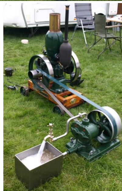
Centre: Dennis Andrew's 1917 Ingeco Type W 3hp owned for 6 years. It was in an old building in Grantham and he received it in payment for helping to clear a shed out. It took 1 year to restore with new parts being made. See picture of unrestored state.
