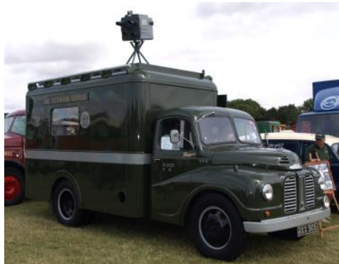
Above: 1955 Austin Loadstar owned by Mr & Mrs B J Morgan since 2009. Nicknamed 'Thumper' because of the noise the generator made when in use. It was originally owned by the BBC and used as a generator lorry for outside broadcasts. It was one of a series of 10 lorries all with consecutive number plates but it is believed to be the only one remaining. It was used for outside transmissions of Sir Winston Churchill's funeral in 1965 and the World Cup in 1966. Used many times before being withdrawn in 1968.
