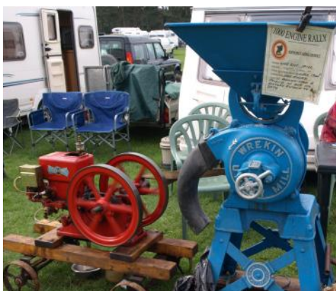
Below: Dave Mycock owns this rare 1922 open crank Worthington Economy 1.75hp running a Welsh Wrekin Mill
