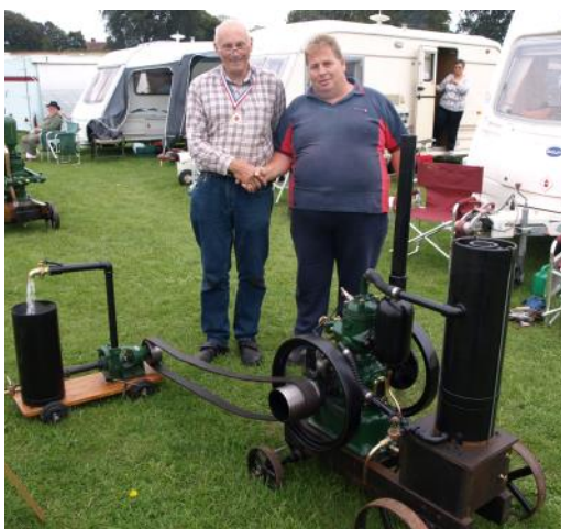
Below: Dave Mycock owns this rare 1922 open crank Worthington Economy 1.75hp running a Welsh Wrekin Mill
