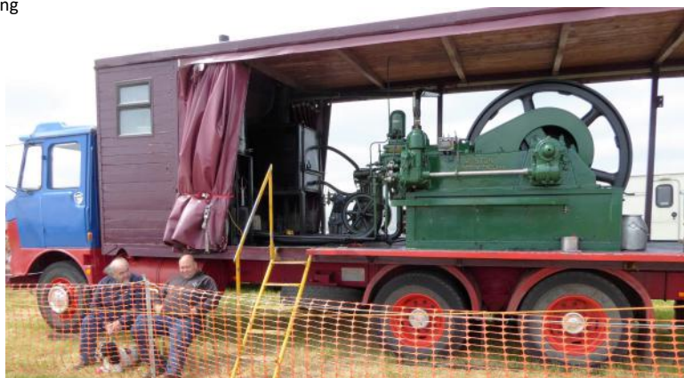
Above: a 1947 Ruston Hornsby 7XHR, 40hp owned by David & Andrew Fox worked a line shaft in the River Board Worksops at Landing Lane, Riccall until 1987.
