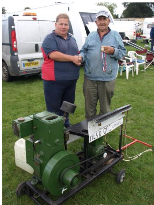
Right: At Holkham 2015 Eddie with his 1945 Lister D that was used to drive a potato shaker. Eddie converted it to drive a dynamo for lighting. I must say 'Eddie, well done for attending with your broken foot!'
