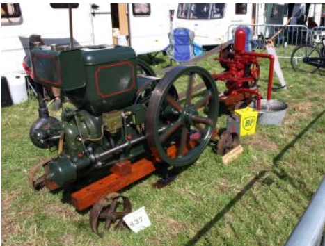
Ruston Hornsby AP 8hp 1924 running a Climax 2 water pump owned by Martin Howell St Neots
