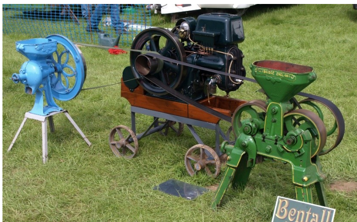
Below: Dean Smith's 1913 Bentall open crank with Bentall roller mill and plate mill
