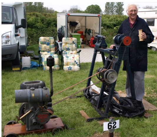
Below: John Woodhead's 1922 Ruston Hornsby model 1P 5hp supplid to Duke & Ockenden Ltd Ferry Wharf Works West Sussex
