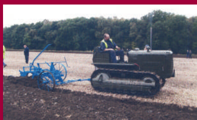
Dorman Engine married to a Cat D4 Running Gear with 2 Furrow Plough.
