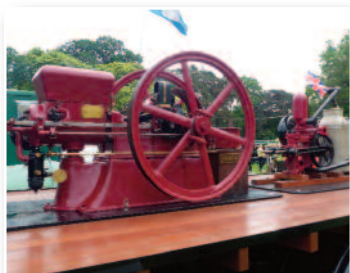
Amanco, 6 horse power 1917, used for pumping water near Doncaster.
