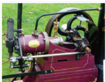
Lovell 1 1/2 horse power 1907, Open Crank Gas Engine, made by the Lovell Company of Boston Lincolnshire. Production of engines ceased around 1915.
