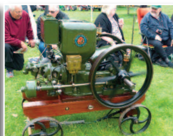
Ruston Hornsby model A.P., 8 horse power 1928. High tension ignition with Wico EK magneto. All petrol.
