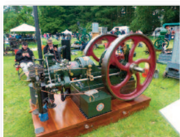
Shanks 12 horse power 1922, made in Arbroth Scotland. Running on heating oil by Hot Bulb Ignition.
