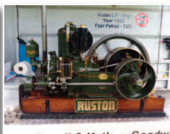
Ruston Hornsby model I.P., 5 horse power 1923, engine number 124873. Low tension ignition, petrol/paraffin.
