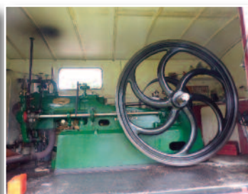
Crossley, type SS 1904, used to operate Crowle Swing Bridge over the Stainforth and Keadley Canal.
