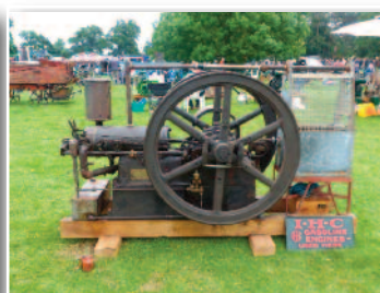
International Harvester Company, 6 horse power 1912, battery and coil low tension ignition, imported from the USA.
