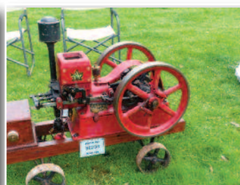
Acadia 2 horse power, approximately 1920, made in Canada, low tension ignition, petrol engine.
