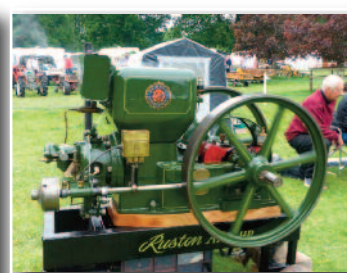
Ruston Hornsby model A.P., 4 horse power 1929. High tension ignition, all petrol. Very nicely lined out in apple green as original.
