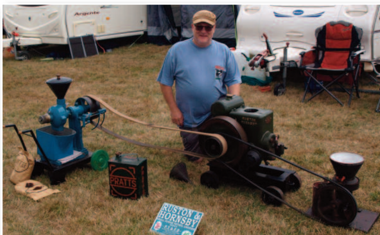
Stacey Burnett with his 1944 Ruston & Hornsby 1.5hp driving a Paint Pigment Mill and a Coffee Mill.
