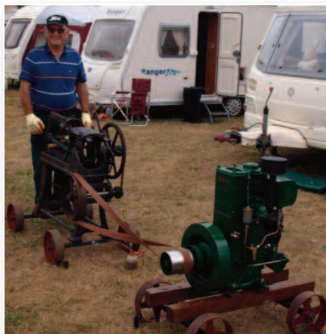
John Bailey with his 1935 Lister D and Rapidor Manchester Power Hacksaw that he was using to cut steel to make wheels for an engine trolley.
