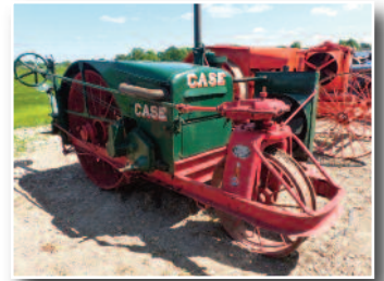
Case 10-20, 1915, 3-wheel layout. The first Case model with the cross motor engine
