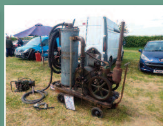
Sturtevant Industrial Vacuum Cleaner Powered by Petter Junior 2 1/2 HP
