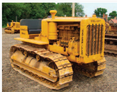
Diesel 40, 1935 Believed to be an original import into South Lincolnshire. Donkey engine start diesel. One that had been restored by Mr. Wilson.
