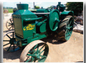
Rumley Oil Pull type 'L' 15-25 H.P., 2 cylinder horizontal engine, oil cooled
