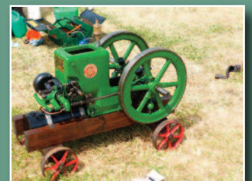
Fuller & Johnson, Type No. 1917, 1 1/2 HP Low Tension Ignition Hit and Miss Engine
