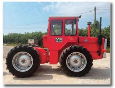
Newark Show also hosted an event to mark the 50th anniversary of the MF 1200 articulated 4WD tractor. This was a very unusual design to the British farmers. It was built at Barton Dock factory in Manchester and was powered by a Perkins 6.354 engine producing 105 hp and weighed around 5 1/2 tons, 2232 were made between 1972 and 1979. It was then replaced by the MF 1250. A fantastic range was on show with original and restored tractors on display.
