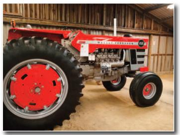
MF 1150, it was built from 1970 to 1972, considered to be a huge tractor at the time it was powered by a Perkins AV8, 510 engine producing 144 hp with a weight of over 5000 kg. It had the luxury of power brakes, power steering, power clutch and power seat. It has a price tag of \$14,000. This model was never officially offered in the UK.
