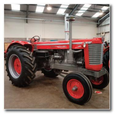
MT 97, this model was sourced from the Minneapolis Moline to fill a gap in the MF product line for high horsepower tractors. It has an unusual engine made up of three blocks of two cylinders producing 112 hp from its 8.3L, it weighed in at 3690 kg. It was on sale from \$6940, sales peaked at 1750 in 1962 it was withdrawn from sale in 1965.
