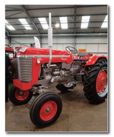
MF Super 90, was produced from 1961 to 1965. This tractor had the option of a Perkins 4.302 diesel engine producing 77 hp or a Continental 4L petrol engine. It also had a independent hydraulic PTO, it weighed in 3280 kg. Some came to the UK for evaluation and one was known to stay in Lincolnshire and worked there for many years, it was later sold at a Cheffins sale for restoration.
