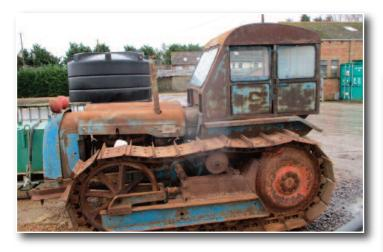
Well things have moved on a pace and I have discovered the crawler was parked up in the farm shed around 1982. Though the water had been drained out this has been her resting place for some 40yrs. After some serious coaching with replenished oil, water, fuel and a tweek or two with the electrics, a sniff of ether and a cough and sputter and away she went.
