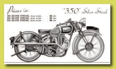
The Silver Streak had high ground clearance and a substantial crankcase shield which made it a good competition motorcycle. A low bottom gear made it useful for cross country and close ratios made it a fast road bike.
