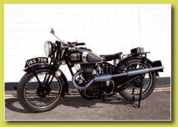
The AJS Silver Streak was a British motorcycle launched in 1938 and described in the sales brochure as the 'aristocrats of the motor-cycle world'. Produced with a choice of 250 cc, 350 cc and 500 cc engines, the Silver Streaks were super sport machines with a special polished finish and hand tuned engines. As many parts as possible were specially chrome plated, including the mudguards, headlamp, fork links, front and rear chain cases, oil and petrol tanks and even the tool-box.
