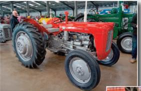
Above pic: this is a Massey Ferguson 42 built in France, much like a MF35 with an MF65 back end with disc brakes, this is a fantastic restoration.
