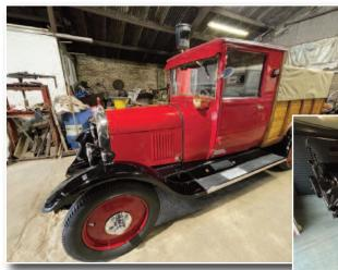
from its 3-speed gear box was 80km per hour which is approx. 50mph. In March of 1927, the B14 was updated with four drum brakes and a servo assistance. The BI4 was
