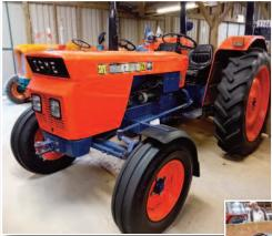
Same Minitauro 60, made in Treviglio Italy an unusual 2 wheel drive version again a lovely restoration. All Same tractors of this period used air cooled engines. They were first imported into the UK in mid 1960s. Right pic: Massey Harris Pony built in Canada from 1947-54 using a continental engine in 1951 production started in France where is was powered by a Simca or Peugeot engine and later with a Hanomag 2 stroke diesel engine.
