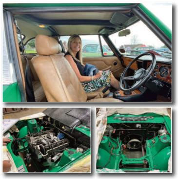
the clutch to line up and even tighter to get all the bell housing bolts in but its in, with the cabs both completely rebuilt and all new pipes and air cleaner we were getting somewhere. Oil in, coolant in, petrol in and we were ready to give her a try. She struck up pretty well and now still six months later seems to start and run just fine.
