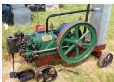
1912 Fielding & Platt, made in Gloucester. Running on propane with Hot Bulb ignition. Fielding and Platt were much better known for their much larger industrial engine.
