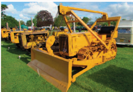
Tom Balls' 1943 Caterpillar R4. An all petrol model with what is believed to be a unique in the UK LeTourneau cable operated blade
