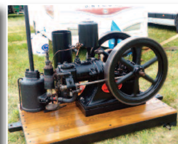
1909 Tange Oil Engine model AA 2 3/4 HP. Originally sold to B.S.A. Ltd., British Small Arms of Birmingham, hot bulb ignition.
