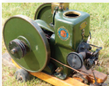
1929 Ruston Hornsby 2 HP ZRP Solid Flywheel model, note the Lincoln Imp embellishment and Wico EK magneto.
