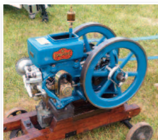
1917 Empire approximately 2 HP low tension ignition.
