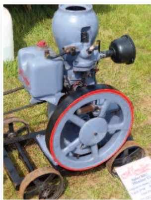
1938 Monitor 1 1/4 HP Petrol Engine imported from the USA with Buzzcoil Ignitor. All joints are taper fit to eliminate the need for gaskets.
