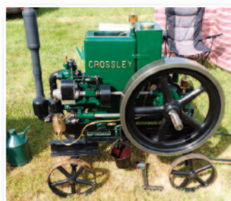
1925 Crossley model 1030, 1 1/2 HP, petrol/paraffin fuel, Enclosed crank horizontal.
